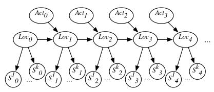
Loc consists of  $(x, y, \theta)$  – position and orientation k = 24 sonar sensors (all very noisy)
