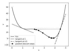
y = 2 \* (x - 1.3) \* (x - 1.5) \* (x - 2) \* (x - 4.5) + 15Step size is 0.05 and gradient descent starts at x = 4.5. What if it starts at x = 5.5? (Hint: the derivative is more than 4 times larger). What if it starts at x = 1.5?
