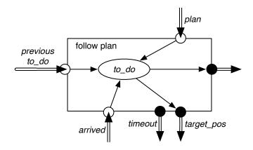
given plan: to\_do := plan timeout := 200 while not empty(to\_do) target\_pos := coordinates(first(to\_do)) do(timeout, target\_pos) to\_do := rest(to\_do)
